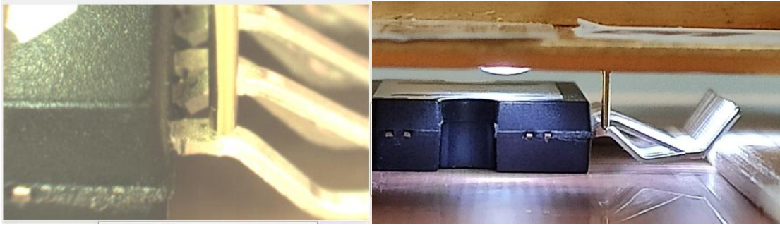
Figure 71: Pogo Pin Landing on Adjusted Lead
